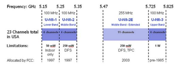
Figure 1 Different sections of the 5 GHz unlicensed band. The FCC in 2014 modified the U-NII-1 rules to allow outdoor transmission at 1 W. Image from [21].
